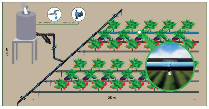
For direct connection to the water mains, we recommend a pressure reducer not included in the package. Kit includes the fittings necessary for the extension to 350 m<sup>2</sup> buying the 100 m Aquadrop reel
